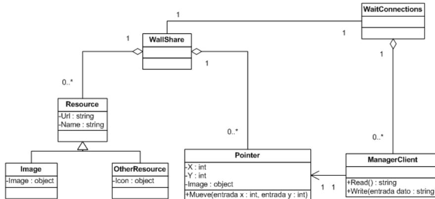
Fig. 4. WallShare class diagram (server side).
